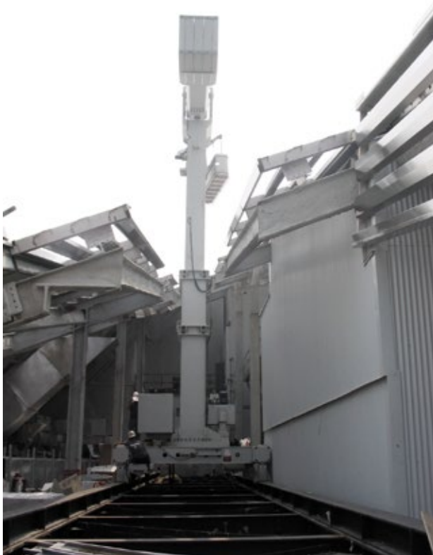
Hydraulically operated telescopic slewing mast
