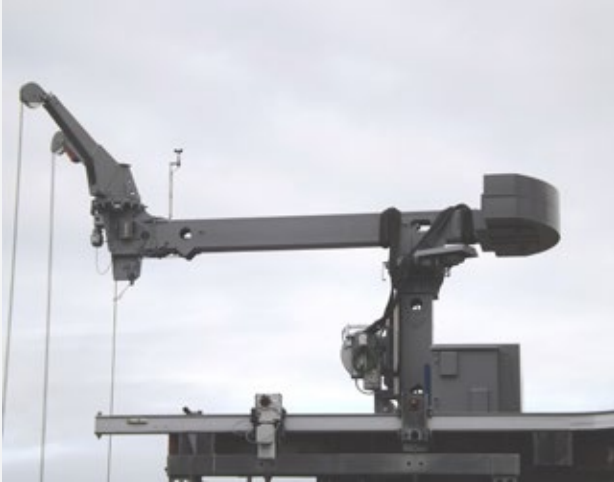
Auxiliary hoist to transport glass panels and facade elements outside the cradle - movable or fixed installation
