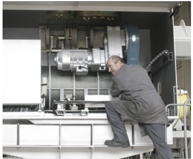
▶ High-performance hoist unit, approx. 4,000kg lifting capacity.
