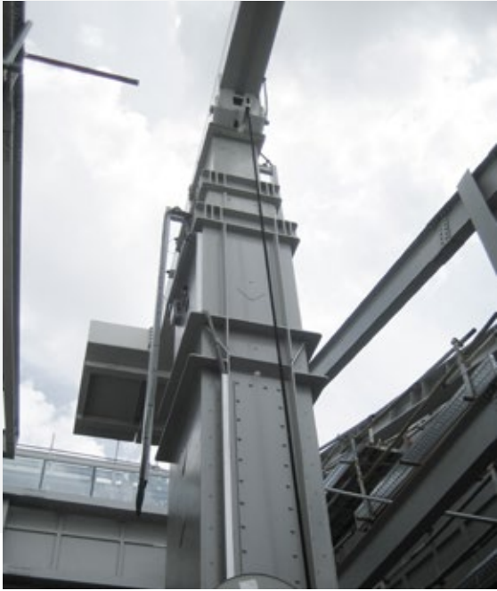
Type 6.4 with telescopic jib and double telescopic slewing mast
