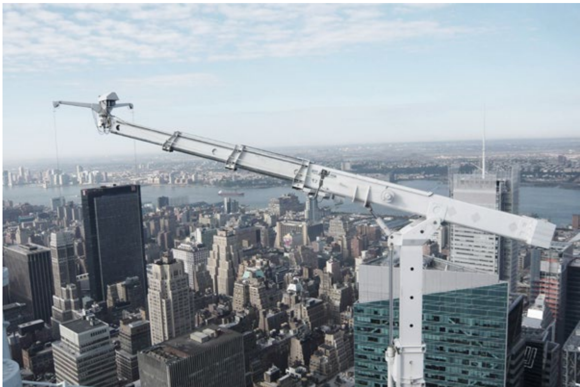
Crane BMU with telescopic jib
