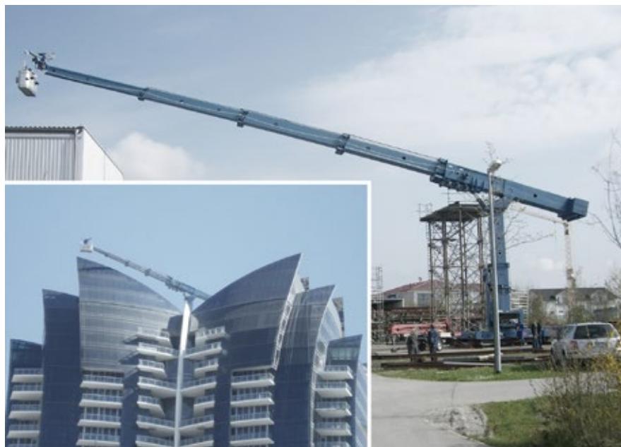
Type 6.4 with a quadruple telescopic jib, slewing device and telescopic mast. Unit assembled at factory for testing and mounted on building roof.
