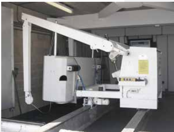
▶ Retractable jib arms for garage/parked position
