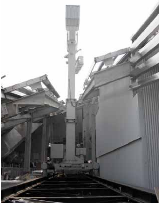
Hydraulically operated telescopic slewing mast
