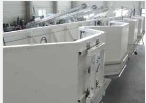
Customised cradle - 15m long for replacing large facade elements
