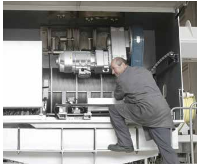
▶ High-performance hoist unit, approx. 4,000kg lifting capacity.
