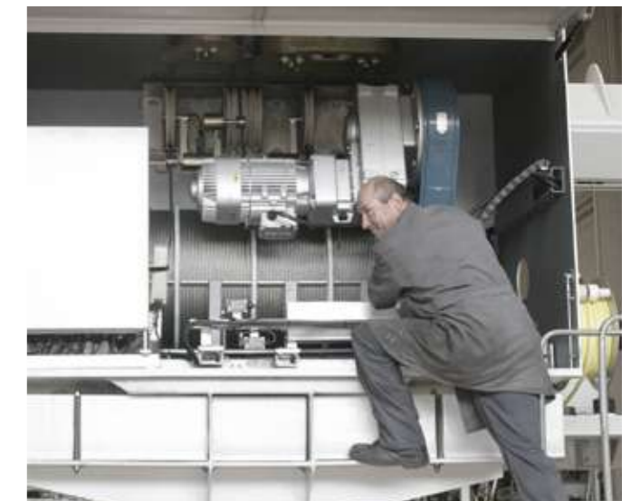
▶ High-performance hoist unit, approx. 4,000kg lifting capacity.
