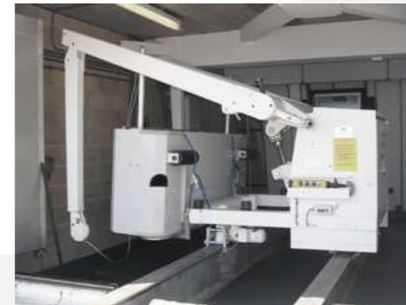
▶ Retractable jib arms for garage/parked position
