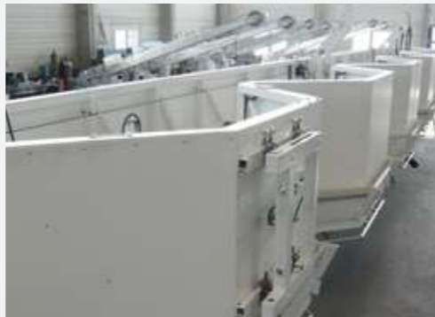
Customised cradle - 15m long for replacing large facade elements
